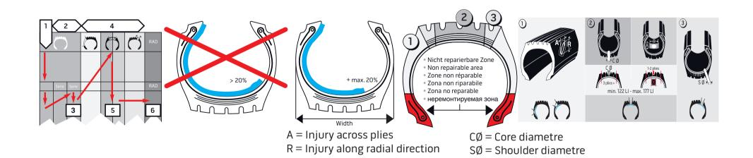
This chart is applicable for tyre repairs carried out within Australia, using REMA TIP TOP repair material and system.
